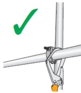
Guardrail on right angle couplers
