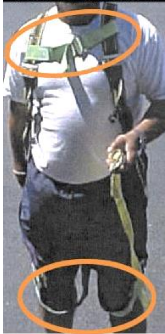
Chest strap positioned too high and too loose. Leg straps are positioned improperly.
