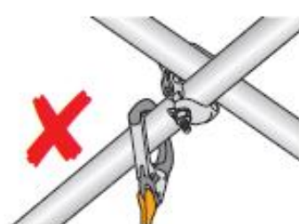
Transoms underslung on non load-bearing couplers
