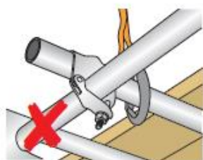
Transoms below foot level
