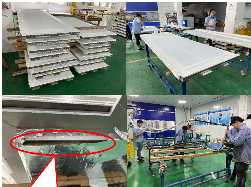
The foil wrap of the thermal insulation foam is damaged is rejected by QC
