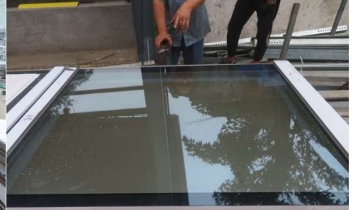
Leakage was found during water flooding test
