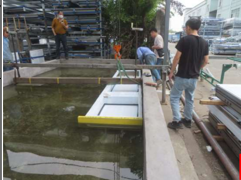
Leakage was found during water flooding test
