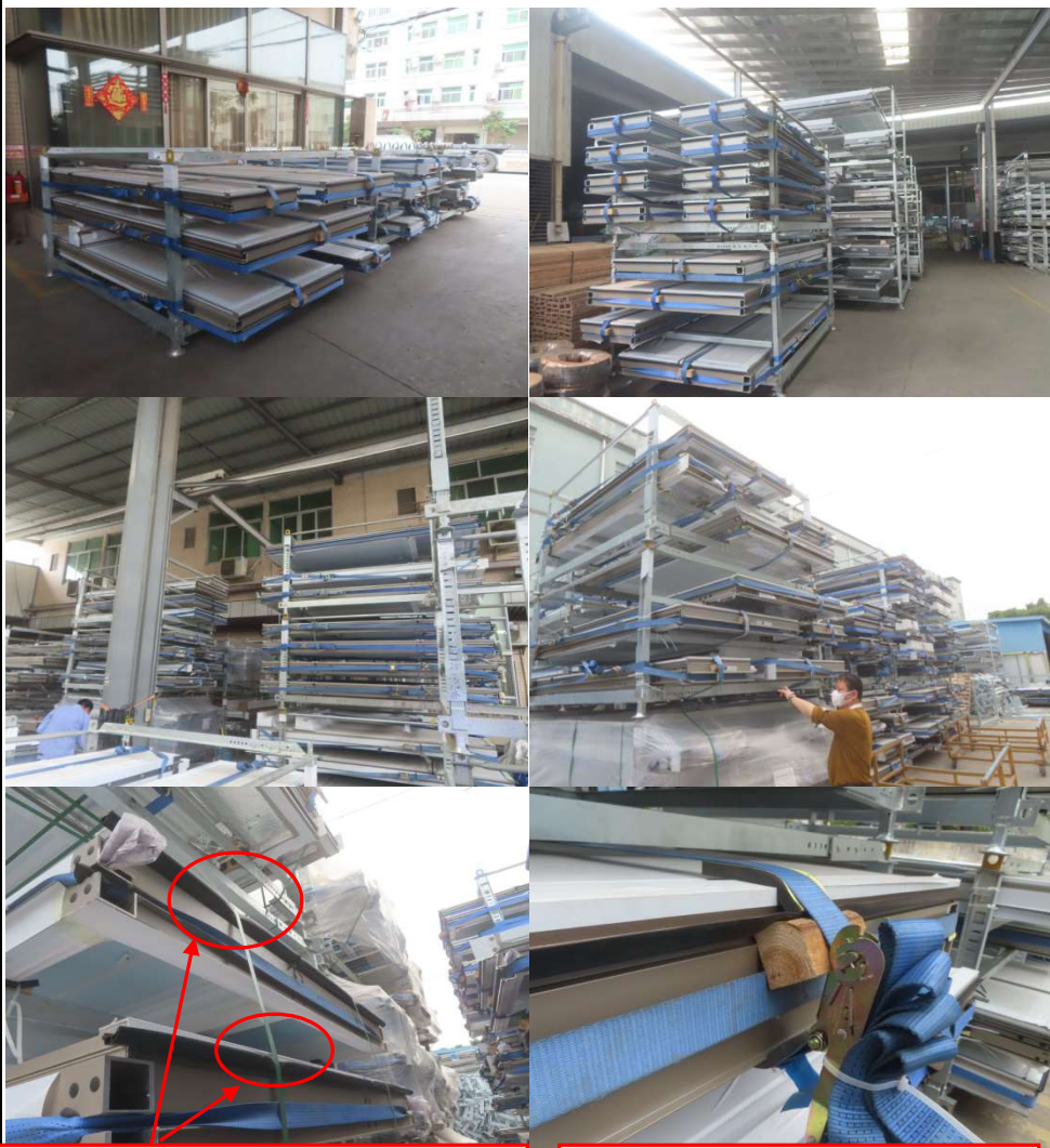
Missing wooden block for protection of gasket
