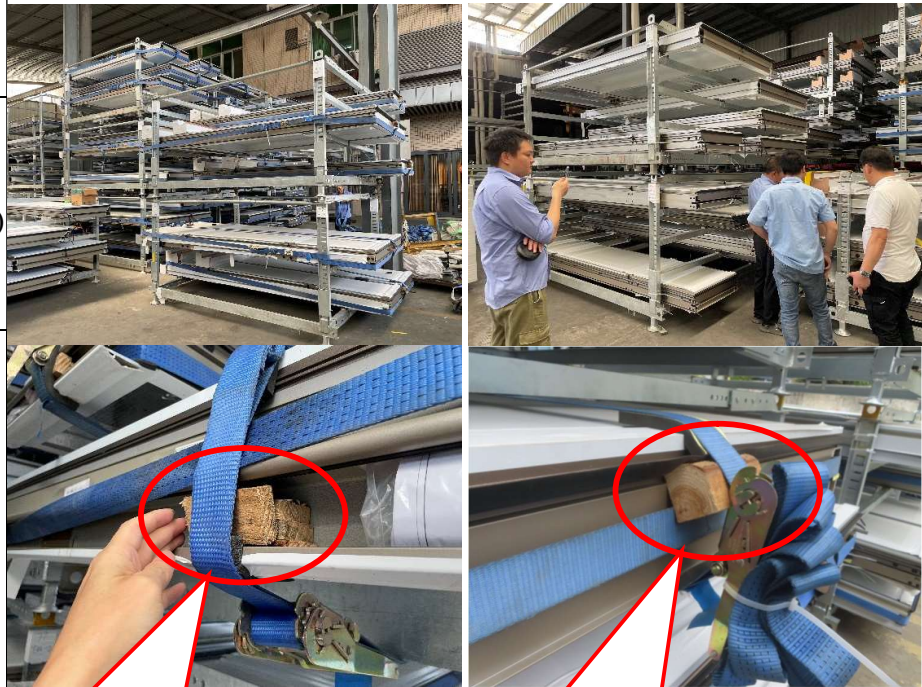
Undersize setting block was found during factory inspection
