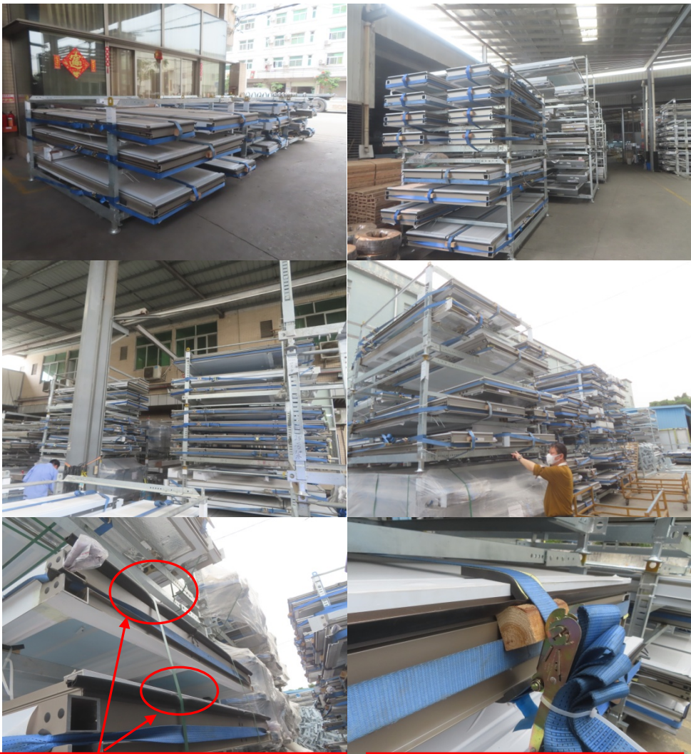
Missing wooden block for protection of gasket
