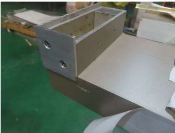
5_Trial assembly of mullion and transom for sliding door
