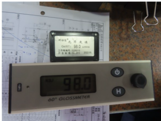
8_Calibration prior test
