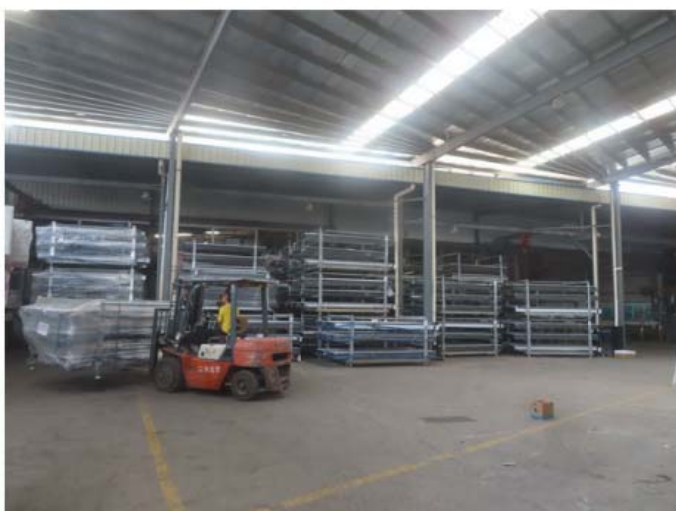
23_Assembled CW panels are stored on the rack
