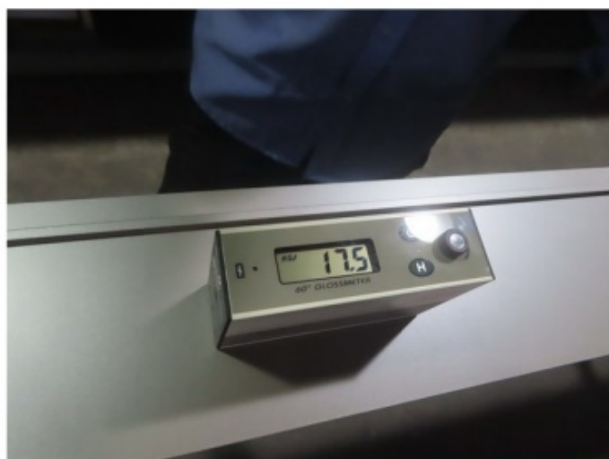
36_Gloss checking by using gloss meter
