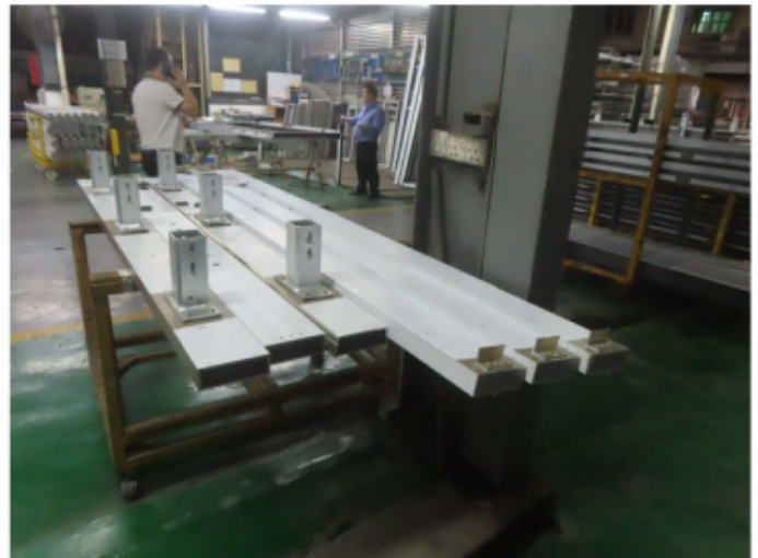
10_Seal-up end position of Transom and Mullion
