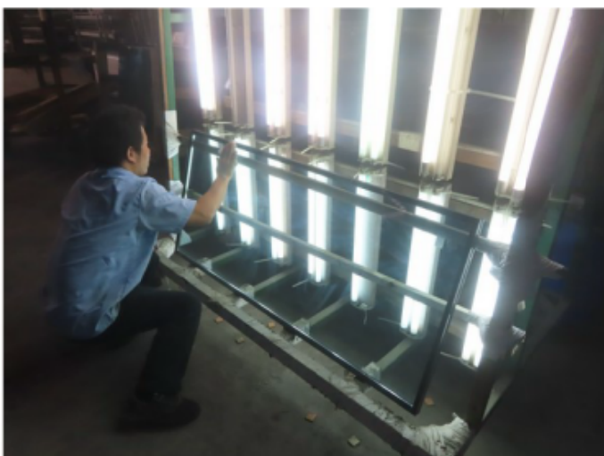
11_QC Checking for glazing
