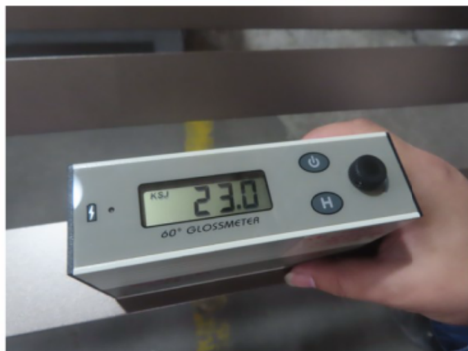
10_Gloss checking by using gloss meter
