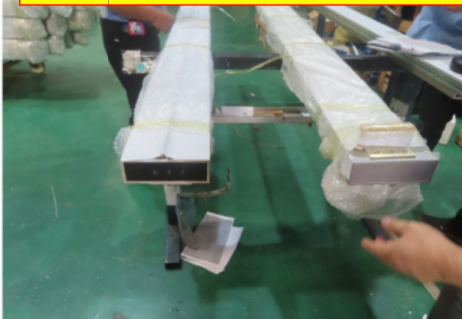
3_ one side of mullion was found concealed
