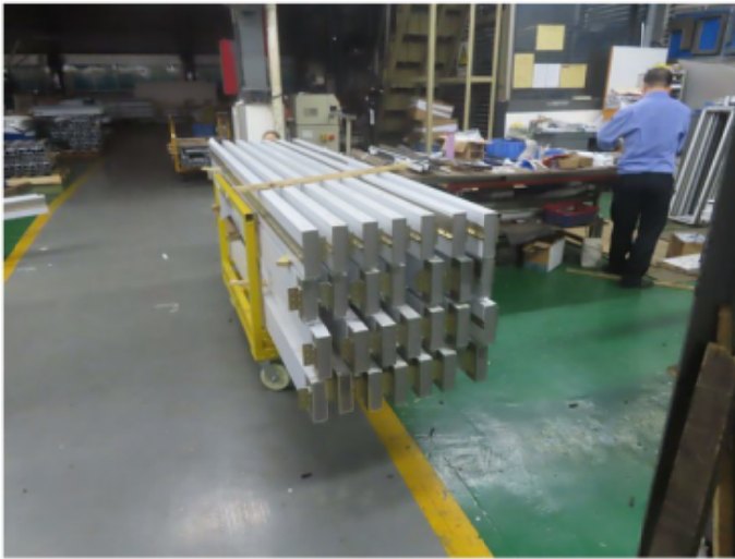
7_Seal-up end position of Transom and Mullion
