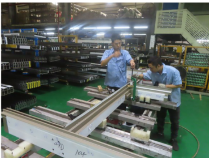
7_General inspection of sealant application at Mullion & Transom interface
