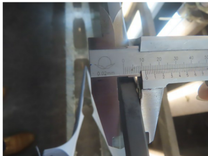
38_Check dimension of Glazing
