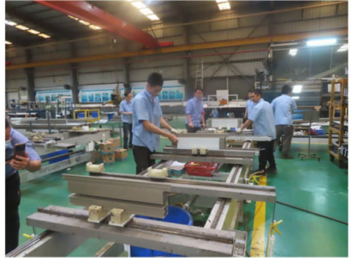
50_Assemble work for mullion and transom.
