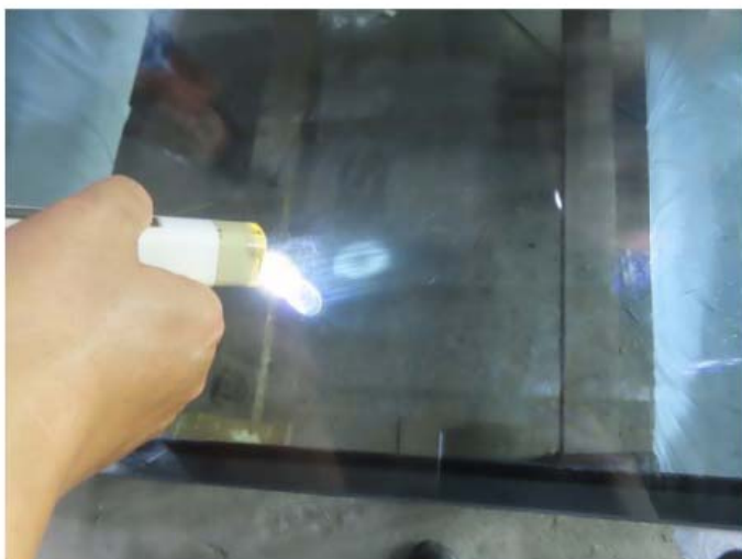
41_Check IGU arrangement and visual inspection
