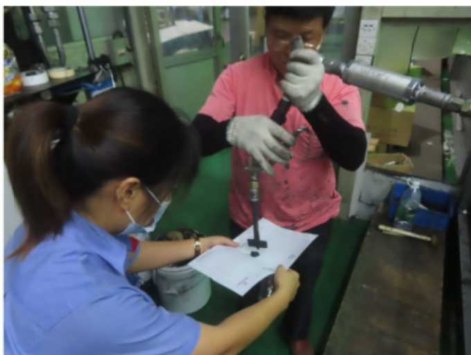
15_ Sampling for structural sealant - Butterfly test
