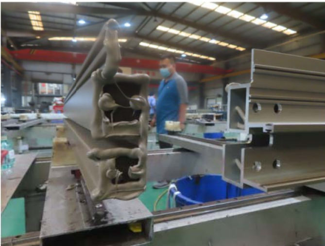
51_Check sealant at mullion and transom interfacing.
