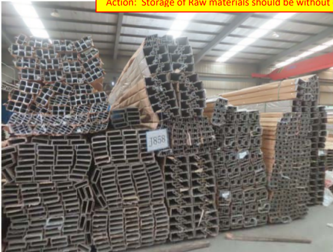
3_Raw materials are in messy and heavy loading condition
