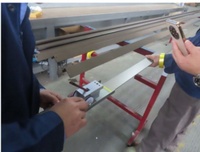
5_Check surface hardness of painting
