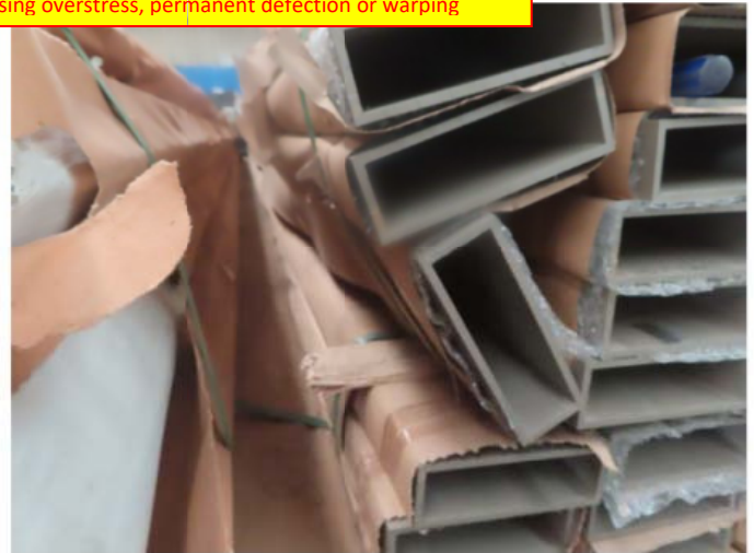
4_Raw materials are in messy and heavy loading condition
