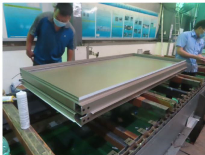
14_ QC checking prior fixing of glazing
