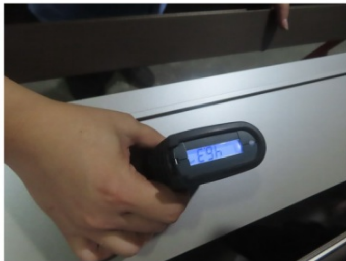
32_ Coating thickness measurement
