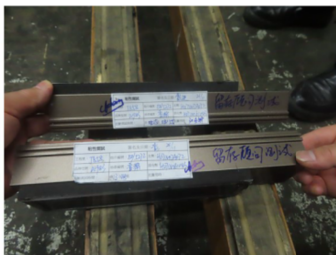
18_ Sampling for Structural sealant - Peel Adhesion test
