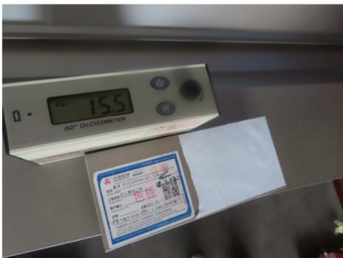
45_Gloss checking by using gloss meter
