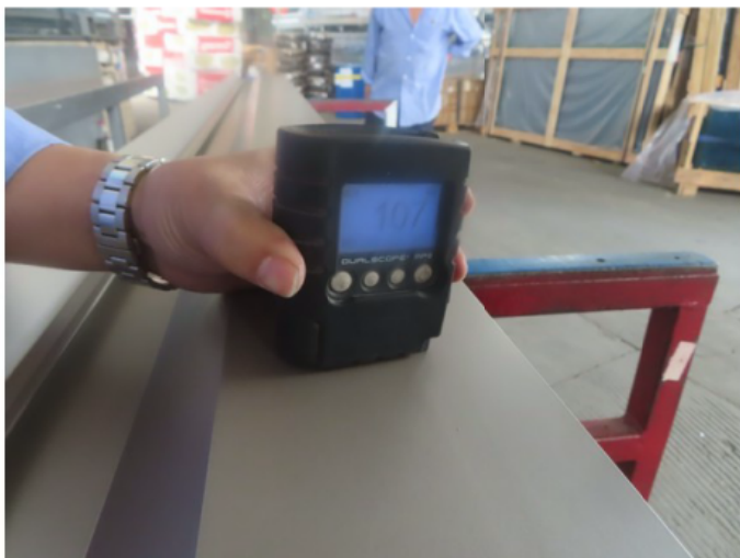
31_Coating thicknes measurement
