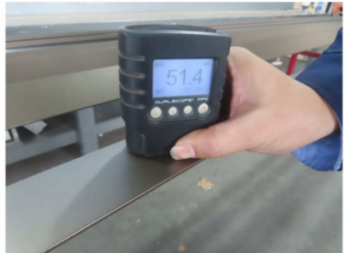
4_Coating thickness measurement
