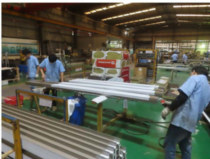
21_Temporary protection prior assembly works
