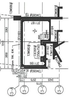
PART PLAN OF DRENCHER WATER TANK NOTE: 1. ALL DIMS ARE (1000x200) BE-SF+0.50, U.N.O. 1 : 100
