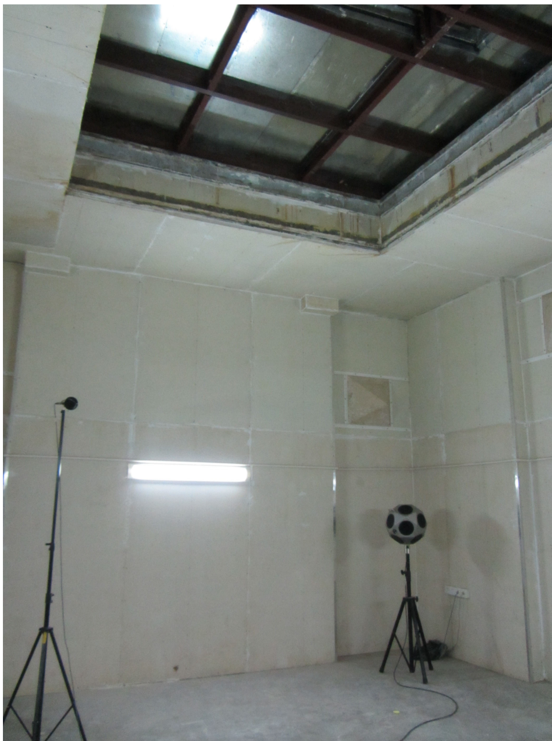
Set-up of Unit Under Test (Receiving room)
