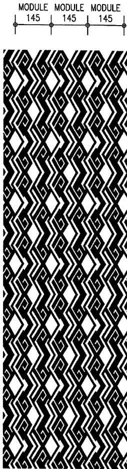
2 ALUMINIUM CLADDING CUTOUT CHINESE PATTERN DETAIL 02
