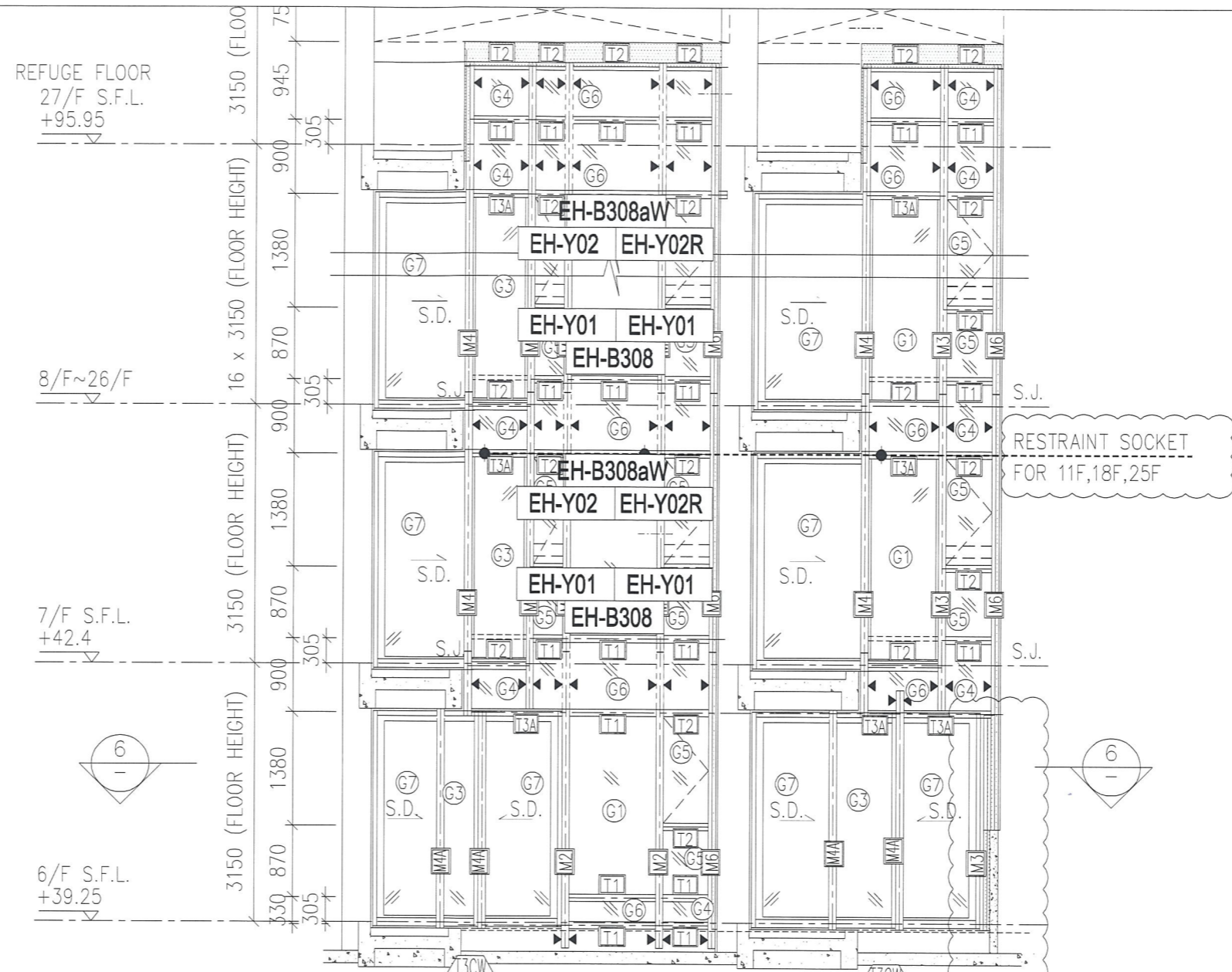
1 - PART ELEVATION FOR CURTAIN WALL
