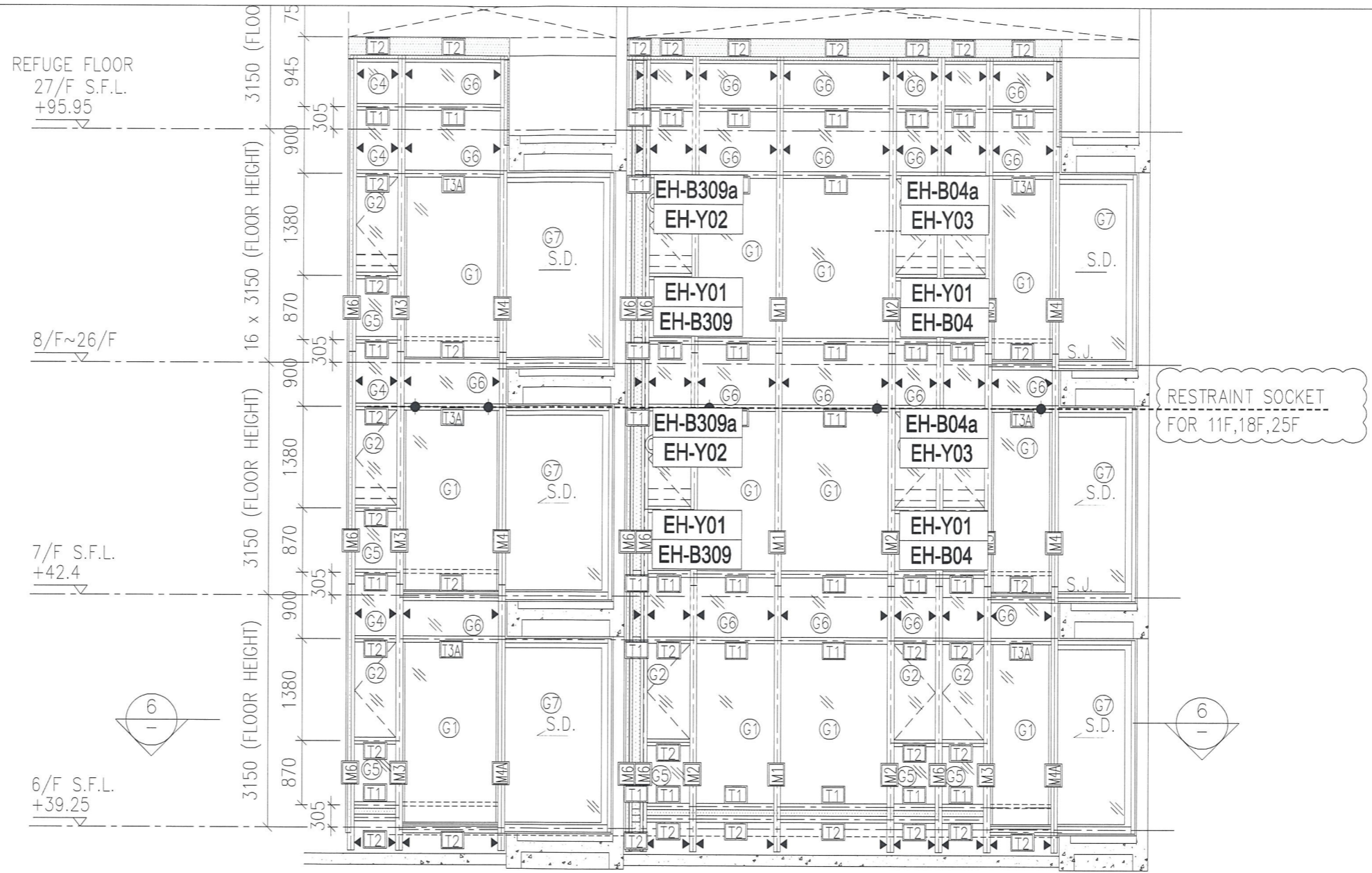
1 - PART ELEVATION FOR CURTAIN WALL
