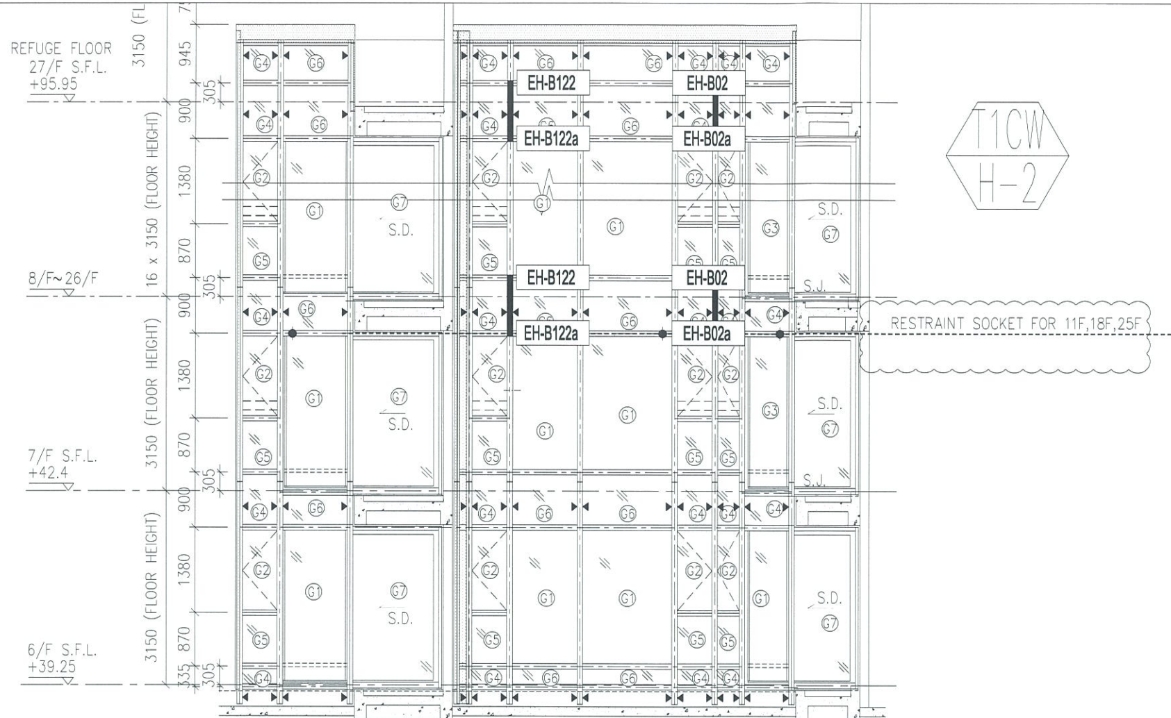
1 - PART ELEVATION FOR CURTAIN WALL
