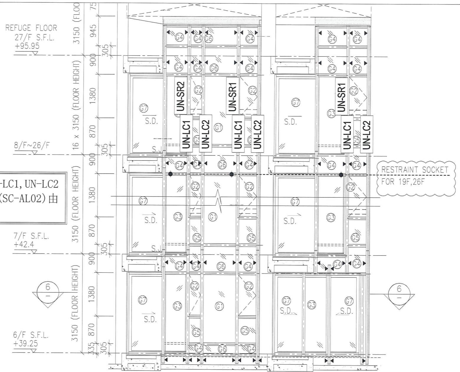
1 - PART ELEVATION FOR CURTAIN WALL
