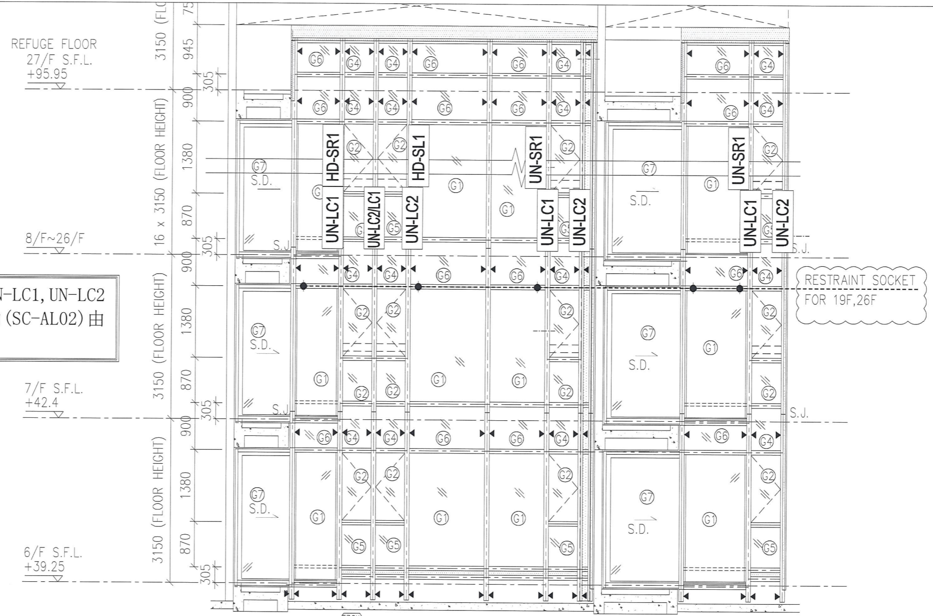
13CW A-1 1 - PART ELEVATION FOR CURTAIN WALL
